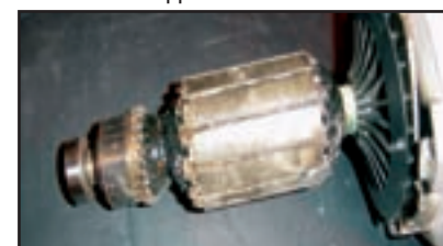
Anker is verbrand (overbelasting)
