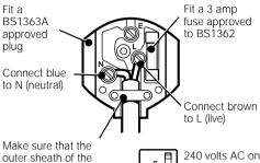
Make sure that the outer sheath of the cable is held firmly by the clamp
