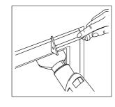
conducted through the metal and can crack the glass. Scrape with the grain of the wood wherever possible. Do not linger on one spot for too long as the surface may char or ignite.
