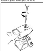
Align the slot of the scraper blade with the protrusion on the blade holder and position under the retaining screw.
