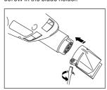
Tighten the retaining screw. Place the blade holder over the nozzle outlet. Ensure it is aligned. The small bump on the inside of the blade
