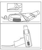
away from you. Secure the cable to prevent pulling your heatgun off the stand. Do not touch the nozzle and ensure that nothing is dropped into the nozzle. Carefully switch off your heatgun and then allow it to cool
