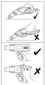
Do not place your hand over the air vents or block these vents in any way. This restricts the airflow through the element and causes over heating. Your heatgun is designed for one-handed use.
