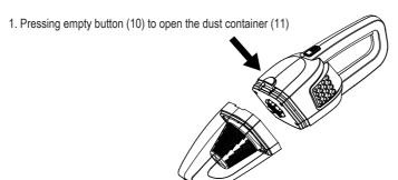
2. Take out the pre-filter (6) and filter (7) together and empty the dust into a dustbin. Return filters and click dust container (11) back into place.
