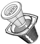
4. Dust container (11) and pre-filter (6) can be shaken clean or rinsed in warm water. The filter (7) can be carefully cleaning by brush, then put into clean water washing. All parts must be dry by airing before reassembled in reverse order.
