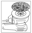
Hold your multi sander with the base upwards. Press the sandpaper disc onto the base, making sure the base is completely covered. It is not necessary to align the holes in the paper and the base. Never use your multi
