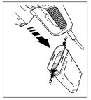
Hold your multi sander vertically with the dustbag facing downwards. Squeeze the sides of the dustbag together, adjacent to the finger grips and pull the bag gently. Empty the dustbag and replace on the sander.
