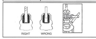
5. DRILLING: Make sure the material to be drilled is tightly fastened and when drilling thin materials use drill at a 90° angle and place enough pressure on the drill for the drill to perforate the surface you are drilling. Never use excessive force when using your drill.
