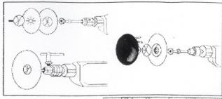
When sanding, do not put all the pressure on the face of the disc; incline the disc at an angle on the surface.
