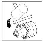
To remove the chuck, open the jaws of the chuck with the chuck key. Hold the chuck firmly in one hand, and with a screwdriver turn the screw set in the chuck clockwise with the other hand until it comes out.
