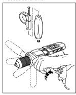
To assemble the side handle, fit the bolt in the clamp and the nut in the handle. Loosely assemble the handle and clamp. Position the side handle on the body of your drill. Rotate the handle around the body of your drill until it is in the desired
