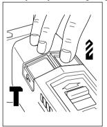
When drilling wood and metal, set the hammer switch to the drill mode When drilling masonry, set the hammer switch to the hammer mode . When screwdriving, set the hammer switch to the drill mode
