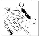
Set the forward/ reverse switch to the desired direction of rotation. Never change the setting of the hammer switch, the speed switch or the forward/reverse when your drill is operating.
