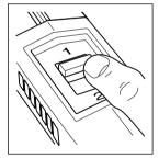
Fit the correct accessory for the job. Set the speed of your drill. On two-speed drills, set the two-speed switch to '1' (low-speed) or '2' (high-speed), or set the variable speed control to the desired speed. As a general
