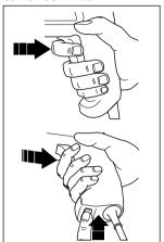
To switch your drill on, depress the on/off switch. Your drill stops when the on/off switch is released. If continuous operation is required, depress the lock-on button while the on/off switch is depressed. To stop your drill when operation is continuous, depress the on/off switch again and release.
