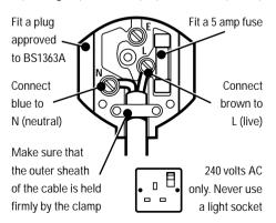
Before replacing the top cover of the plug ensure that the cable restraint is holding the outer sheath of the cable firmly and that the two leads are correctly fixed at the terminal screws. If the fuse cover is missing or damaged do not use the plug. For replacement or detachable fuse covers, contact a Black & Decker service centre.
