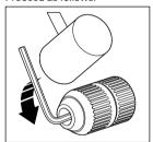
To remove the chuck, open the jaws, hold it firmly in one hand and with a screwdriver held in the other hand, turn the set-screw in the chuck clockwise approximately one turn, to loosen it. Place an allen key in
