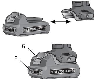
To remove the battery pack from the tool, press the release button (G) and firmly pull the battery pack out of the tool handle. Insert it into the charger as described in the charger section of this manual.
