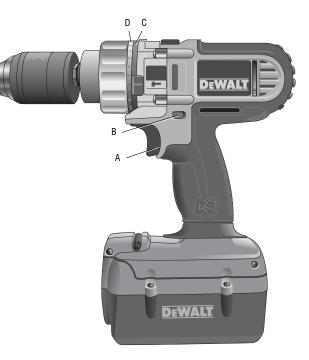
To select reverse, depress the forward/reverse control button on the left side of the tool. The center position of the control button locks the tool in the off position. When changing the position of the control button, be sure the trigger is released. **NOTE:** The first time the tool is run after changing the direction of rotation, you may hear a click on start up. This is normal and does not indicate a problem.
