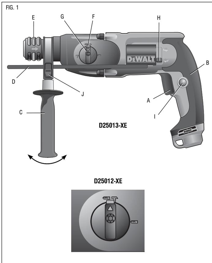
3. Tighten the side handle by turning it clockwise.
