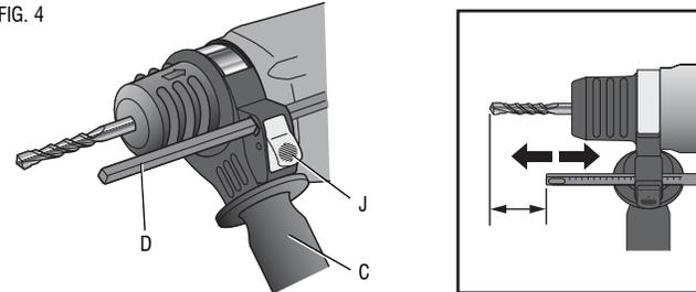
3. Release the button to lock rod into position. When drilling with the depth rod, stop when end of rod reaches surface of material.
