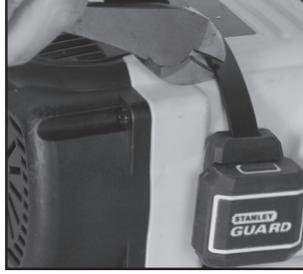
Cutting the tie-wrap of a tool tag
